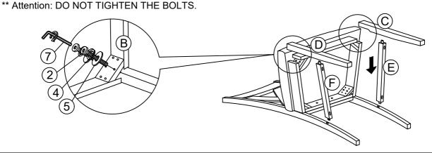
STEP 4: Assemble the stretcher (E & F) by using screwdriver with screw (6).
