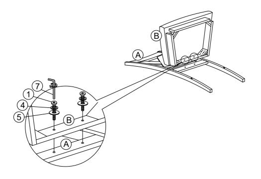
STEP 2: Assemble the Seat Frame (B) with the back legs of Backrest (A) by using Allen key (7) with hardware 3, 4, and 5.
