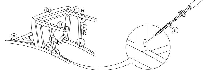
STEP 5: To level the chair ,stand the chair up on a flat surface and tighten all the bolts by using Allen Key (7) and all the screws with a screwdriver.
