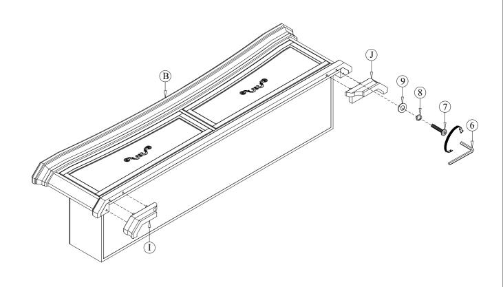
STEP 4 Assemble the footboard support leg (K) to storage footboard (B) by using allen key (6) with hardware 10, 11, 12
