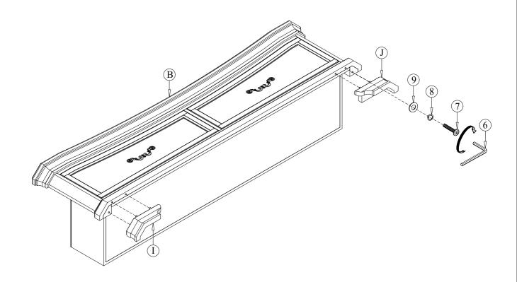
STEP 4 Assemble the footboard support leg (I)to storage footboard by using allen key (6) with hardware 10, 11, 12
