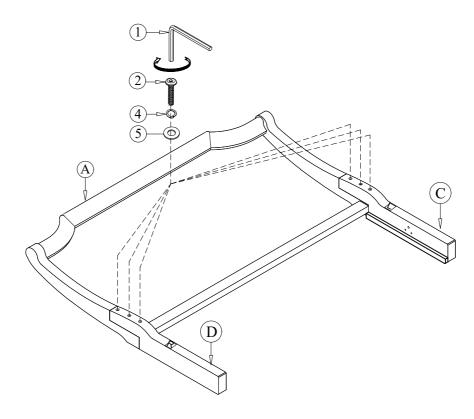
STEP 2 Assemble the headboard cross bar (E) to headboard legs (C & D) by using Allen Key (1) with hardware 3, 4, and 5. \*TIGHTEN ALL THE BOLTS BY USING ALLEN KEY (1)
