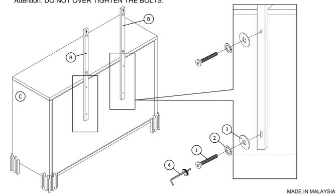
STEP 2: Assemble the Mirror (A) with the Mirror Support (B) by using Allen Key (4) with hardware (1), (2) and (3).
