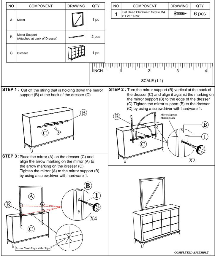
NOTE : MUST TIGHTEN SCREWS PERIODCALLY WITH USE SCREW WILL BECOME LOOSE CHECK TIGHTNESS OF ALL SCREW EVERY 6-8 WEEKS.
